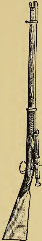
Fig. 68. Whitworth Military Rifle with Davidson Telescope.
